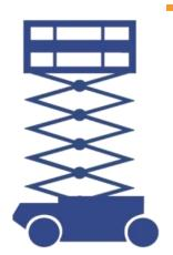
Each MEWP that is designed for outdoor use has a maximum wind speed that it may be used in. This maximum speed is for gusts, so make sure those maximums are not exceeded. Scissor lifts are limited to below 25 MPH, and all lifts will have their maximum wind speed listed in the manual.
